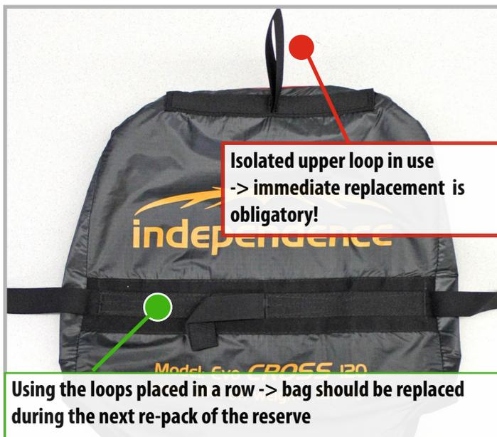
If one of the **three loops in a row**, which are placed between the labellings, is in use, the deployment bag does not necessarily need to be replaced. **These three loops don't show any faults and are not concerned by this safety note** (see image on the left).
